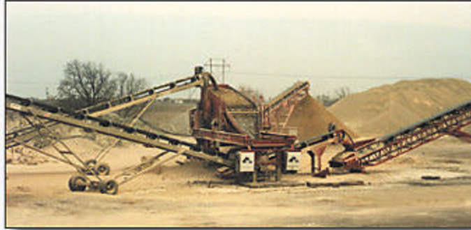
Central Paving began producing RAP and recycled concrete with a Pioneer 4030 Recycler (portable HSI crushing plant) and a Kolberg Model 241 Screening Plant. After the company purchased a quarry, they added a Pioneer CS 2436 jaw crusher and upgraded the Kolberg Model 241 screening plant with a Pioneer 5 x 16 screen.
