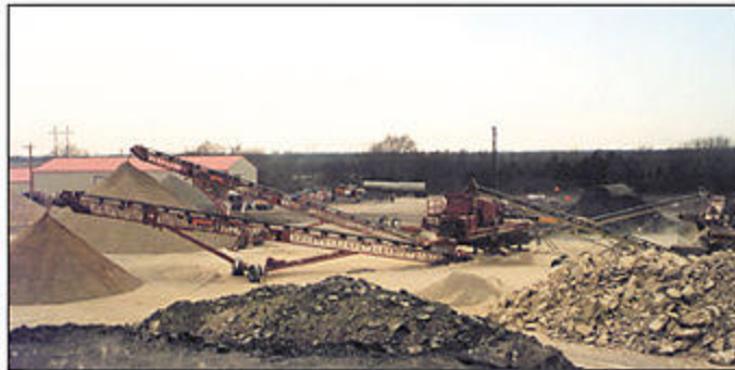
Central Paving purchased portable equipment that could travel with its asphalt plant. On a closed circuit, the Pioneer 4030 Recycler is used as a secondary crusher, or it can be used as a stand alone plant configuration to crush RAP or recycled concrete.
