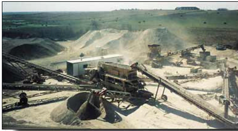
Gratech first screens material and then runs it through a twin jaw. After screening it a second time, material goes to both the VSI and a cone.
